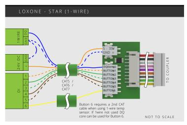
For Loxone systems that have been star wired the FLY-LOXO2 allows direct connection to a CAT cable. It includes a 1-wire temperature sensor. It can be used for 1-6 button keypads.
