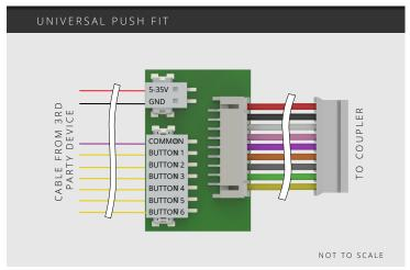
For systems that require a female terminal the FLY-UNIV2 allows the connections of fly leads from any 3rd party device. Supports keypads with 1 - 6 buttons..
