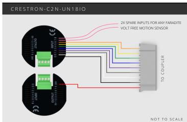
The Crestron C2N-UNI8IO allows for up to 8 inputs to be connected. The supplied Faradite fly lead uses inputs 1 - 6 with inputs 7 and 8 spare for external sensors such as the Motion Sensor 360 - Volt Free. Please note: This module does not support fast double click functions, only use single click functions.
