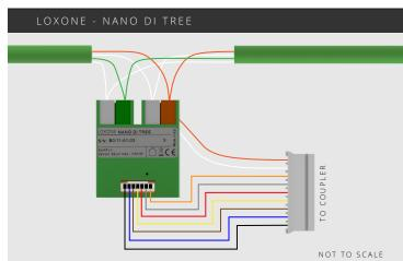
Connecting the TAP Volt Free Coupler to a Loxone Tree bus is simple using the Nano DI Tree. Power the Coupler by connecting the loose orange and white fly leads to the orange and white terminal block.
