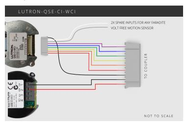
The Lutron QSE-CI-WCI allows for up to 8 inputs. Use the Faradite FLY-LUTR1 to connect the TAP Coupler Volt Free to the Lutron QSE-CI-WCI. Inputs 7 and 8 can be used for additional sensors such as the Faradite Motion Sensor 360 Volt Free.
