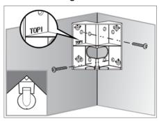
Fix the sensor body to the base plate securely through its own mounting screws and finally adjust the position of the sensor head.
