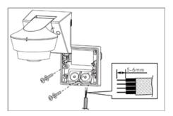
At this point it is recommended to carry out the commissioning of the device (see "Commissioning"), or at least the download of the physical address, using the programming button placed close to the bus connector; alternatively, programming mode can be activated later when the device is already installed by means of the EK-QR6-IR remote controller. Fix the sensor body to the base plate securely through its own mounting screws and finally adjust the position of the sensor head.
