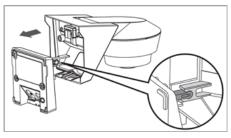
Mount the base plate on the wall / ceiling in the desired position by means of the supplied screw anchors. Drive the incoming bus cable through the rubber perforation cable guides and connect the device.
