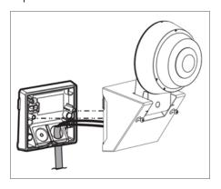
The sensor head can be adjusted up to 40° downward and 90° upward, and rotated horizontally max. 90° in either direction.
