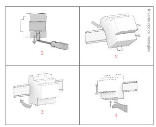
Before removing the device, be sure the inputs have been disconnected and the bus terminal has been extracted from its slot. Use a screwdriver to slide down the locking device and remove the device from the rail.
