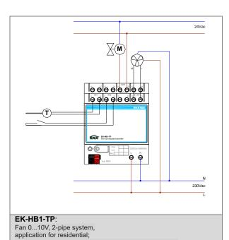
actuator valve for exchange battery powered at 24 Vac
