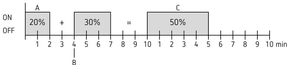
**i** If the rated turn-on time for the current cycle has already exceeded while receiving the new actuating value, the output is immediately switched off and the new actuating value is executed during the next cycle.
