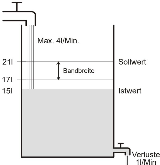
If the filling quantity is 15 l, there is a control deviation of  $21\text{ l} - 15\text{ l} = 6\text{ l}$
