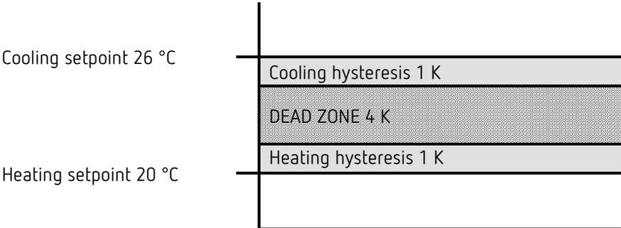
The dead zone (4 K) is increased by the value of both hysteresis (2 K) and offsets the cooling setpoint to 26 °C.
