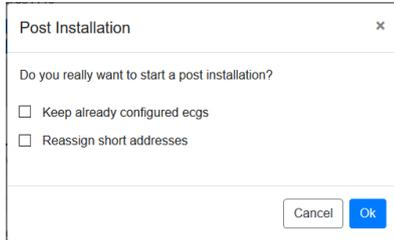
Usually, ECGs have no short address and long address 0xFFFFFFFF on delivery by default. It might be possible, that ECGs got a short address even if long address is still 0xFFFFFFFF (i.e. if an external tool was used for programming). In order to delete short address in this case please activate the control element "Reassign short address".
