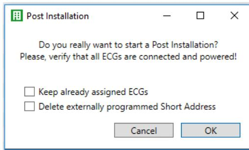
Usually, ECGs have no short address and long address 0xFFFFFFFF on delivery by default. It might be possible, that ECGs got a short address even if long address is still 0xFFFFFFFF ( i.e. if an external tool was used for programming). In order to delete short address in this case please activate the control element "Delete externally programmed short address".
