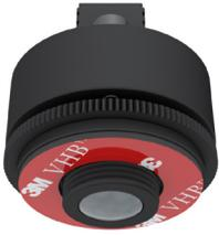
The Faradite Motion Sensor 360 Pinhole - Volt Free is a rear panel mounted, ultra discreet passive infrared motion sensor. It's designed for use with home/building/lighting control systems that have volt free / dry contact inputs.
