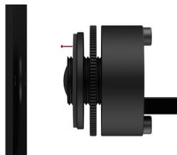
2) Remove the 3M adhesive plastic cover and mount the sensor to the rear of the installation surface. Ensure the sensor is flush to the surface front.
