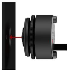
3) Twist the locking nut up against the depth nut to secure the sensor.
