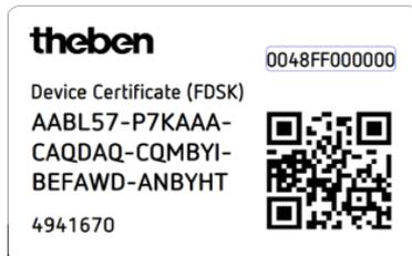
After entering the FDSK, the ETS generates a device-specific tool key. The ETS sends the tool key to the device to be configured via the bus. The transmission is encrypted and authenticated with the original and previously entered FDSK key. Neither the tool key nor the FDSK key are sent in plain text via the bus.
