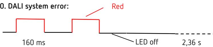
No DALI device is connected to the master, or a DALI line is interrupted.
