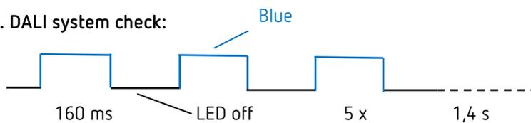
The master checks all DALI devices connected to the DALI bus.
