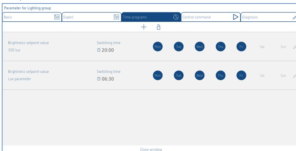
During the night from 8:00 p.m. to 6:30 a.m., the brightness setpoint is reduced to 350 lux. Every working day from 6:30 a.m. to 8:00 p.m., the brightness setpoint (500 lux) is changed to the set parameter value in BASIC. At the weekend, the brightness setpoint remains at 350 lux all day.
