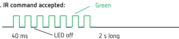
LED flickers (12.5 Hz) when a valid remote control command is received.
