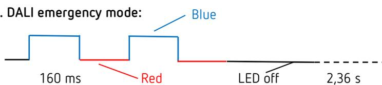
DALI devices have not yet been assigned to a group. The flashing stops when all DALI operating devices have been assigned to a group.
