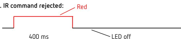
Rejection pulse when an invalid remote control command is received.
