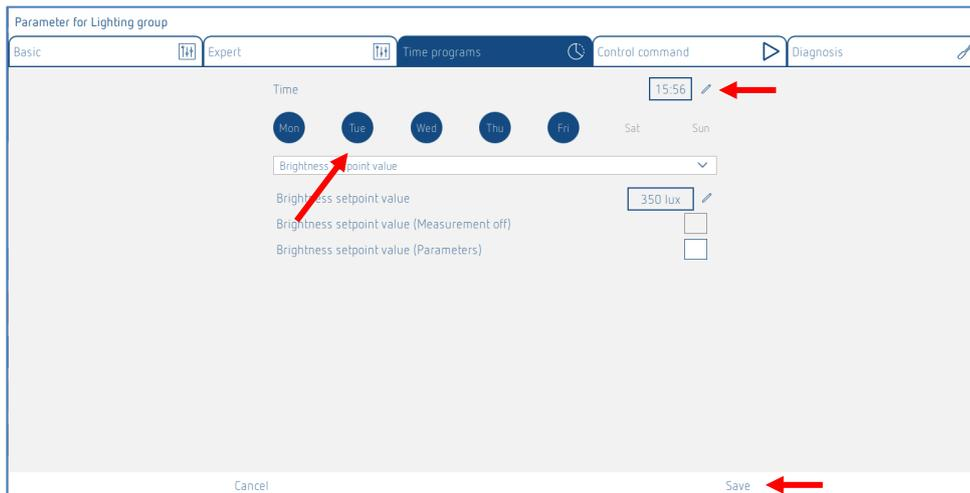
The desired day of the week can be selected by tapping and the time can be entered. The time program record is created by pressing the "Save" button.
