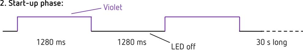
After triggering the restart, the master goes through the start-up phase. This is indicated with this flashing pattern.
