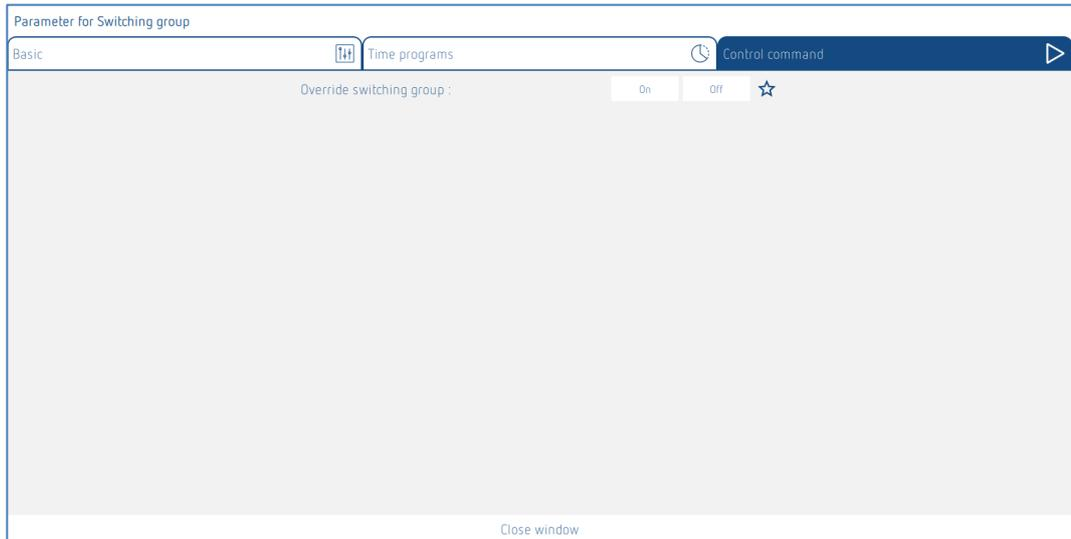
Manual override of the switching group. This override is active until an action is carried out again by push button, scene or time program.
