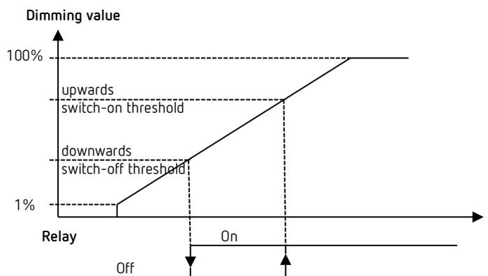
With the factory settings "Upward switch-on threshold = 1%" and "Downward turn-off threshold = 0%", the relay switches on at dimming value 1% and switches off at dimming value 0%.
