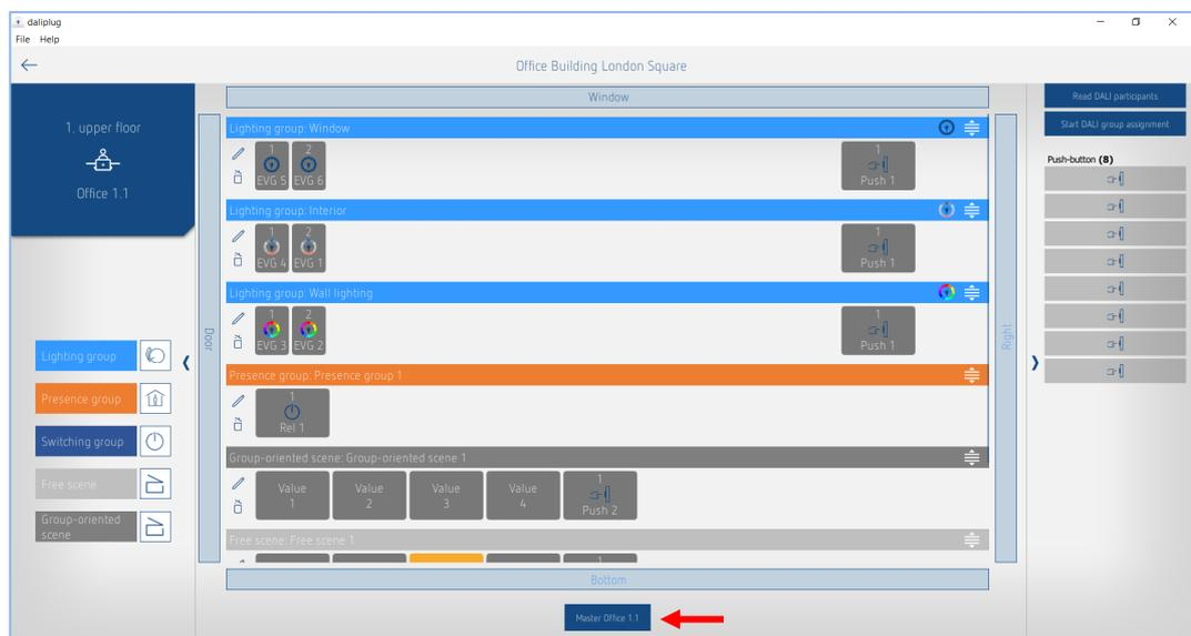
The parameters are accessed by tapping the master. The master must already be connected with the app!
