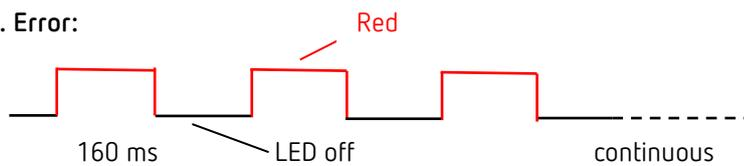
Error flashing (applies until the error has been resolved).
