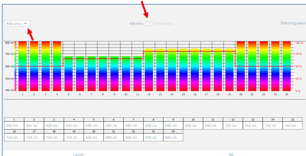
The drop-down menu can be used to switch between the RGB colour curve and the white component curve:
