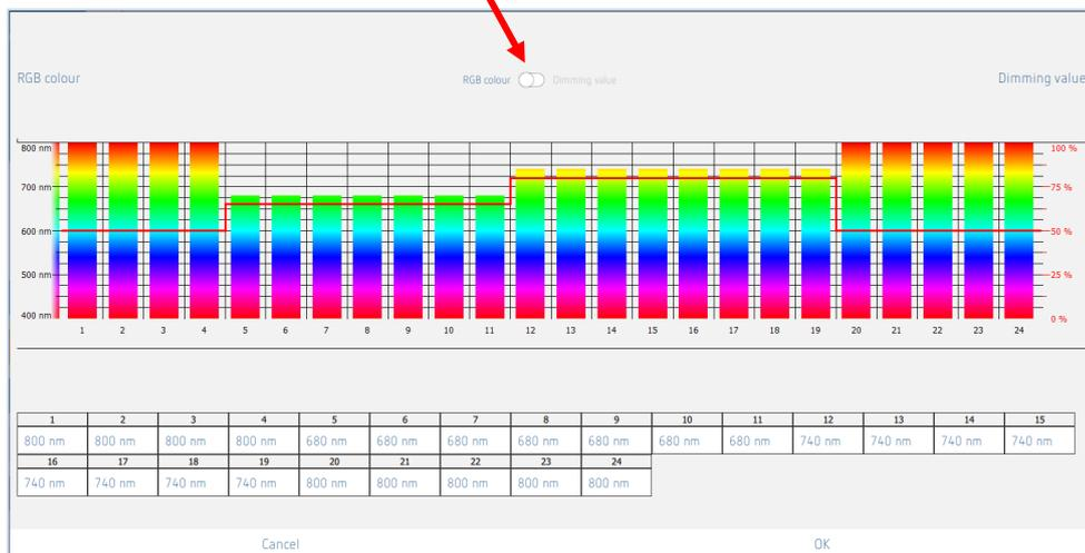
Colour gradient and dimming values are set as desired by dragging the bar in the diagram or by entering the values in the table.
