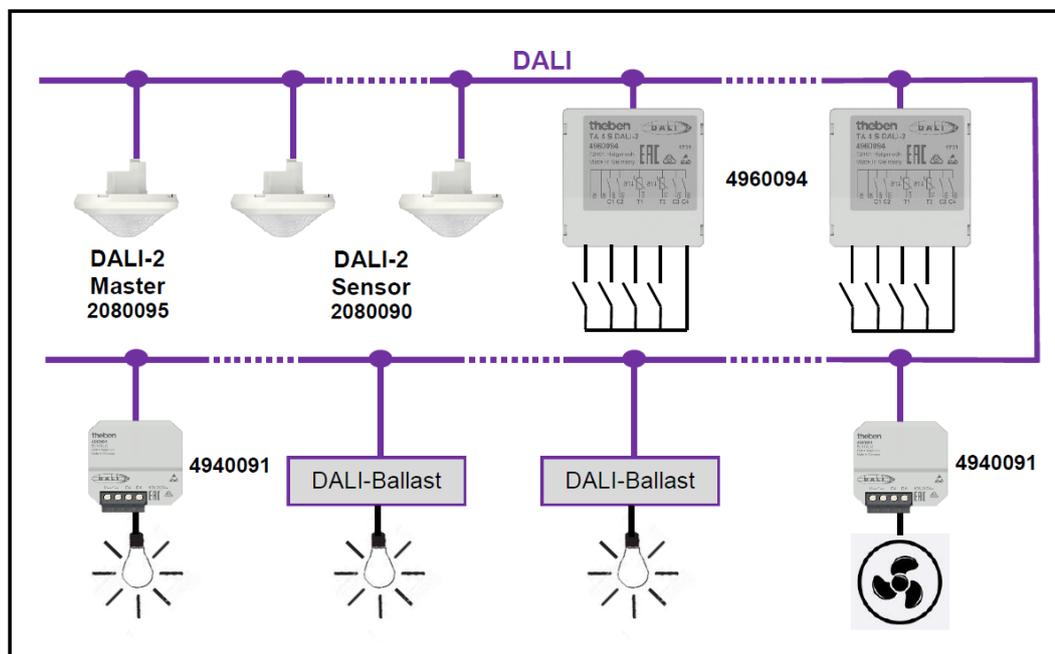
The presence detector theRonda P360 DALI-2 HCL and other DALI components are connected to the DALI line. The DALI supply is provided by the master.
