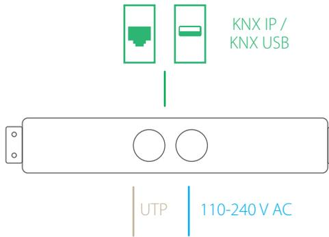
1. **Plug-in** the power supply and connect your Sledgehammer to the network via the network cable.
